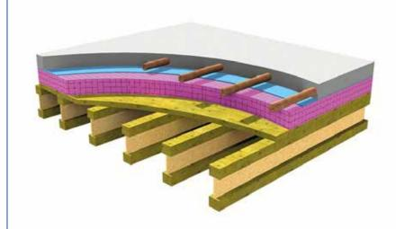
40mm (allow minimum 25mm cover to pipes) of GYPSOL TimBRE Screed with embedded underfloor heating
